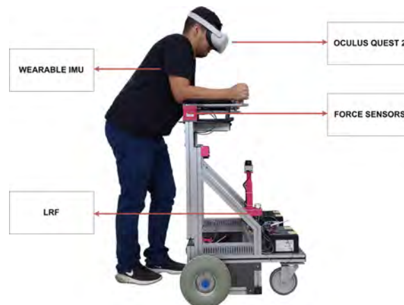
Figure 1: The UFES vWalker and the Oculus Quest 2 being used during a task.
