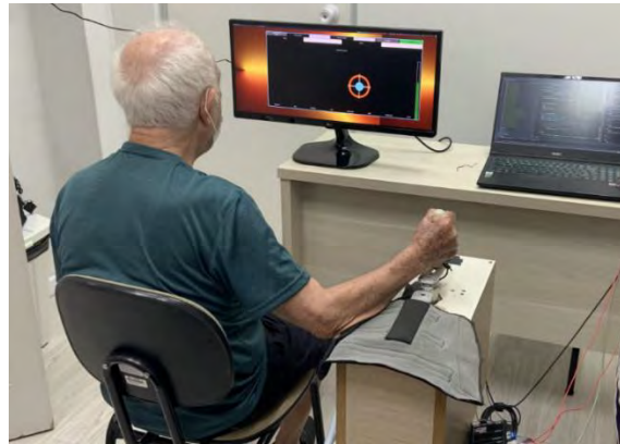
Figure 1. The volunteer hand holds the robotized handle device for the wrist, designated MORE-W. This embedded system is used for measurement of kinetic quantities related to wrist movements.
