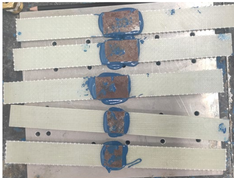
Figure 1 - GRFP repaired with bounded metallic patch
