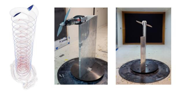
**Objectives.** The research goal is to assess the Aerodynamic and Aeroacoustic characteristics of wings with Distributed Propulsion features, including leading-edge propellers and wingtip-mounted propellers. This configuration poses many challenges as propeller-propeller and propeller-wing interactions are both expected to influence aerodynamic forces and noise levels. The applicant may work with the following fronts:
